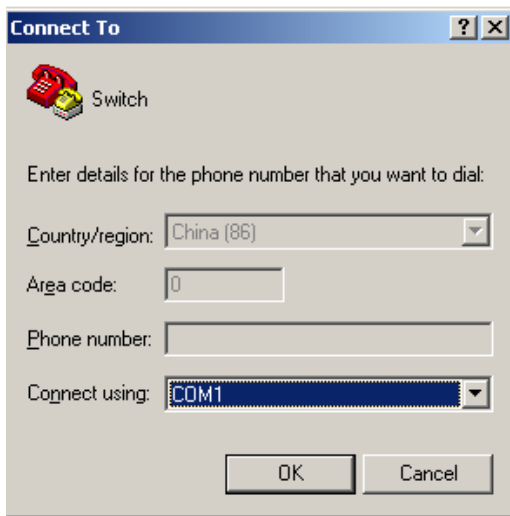
Figure 100 Specifying the connection port
