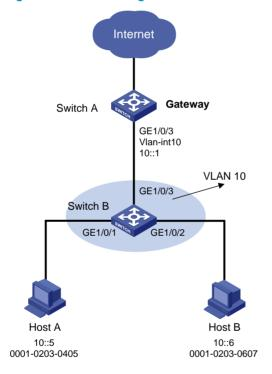
As shown in Figure 94, Switch A serves as the gateway. Switch B connects Host A and Host B. The hosts can obtain IPv6 addresses only through SLAAC. Configure SAVI on Switch B to bind the addresses assigned through SLAAC and permit only packets from the bound addresses.
