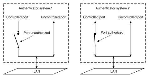
In the unauthorized state, a controlled port controls traffic in one of the following ways:
