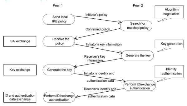
As shown in Figure 55, the main mode of IKE negotiation in phase 1 involves three pairs of messages:
