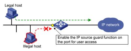
A binding entry can be statically configured or dynamically added.
