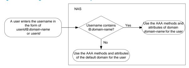
The authentication, authorization, and accounting of a user depends on the AAA methods configured for the domain to which the user belongs. If no specific AAA methods are configured for the domain, the default methods are used. By default, a domain uses local authentication, local authorization, and local accounting.
